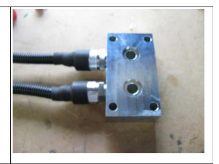
ALWAYS use HYDRAULIC THREAD SEALANT on the pressure sensor threads. NEVER use Teflon based products.
